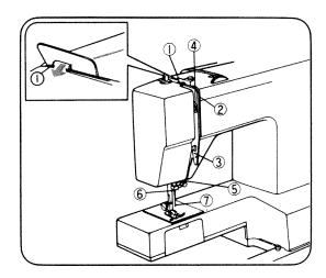
Lead thread either side of tension disc ②.
